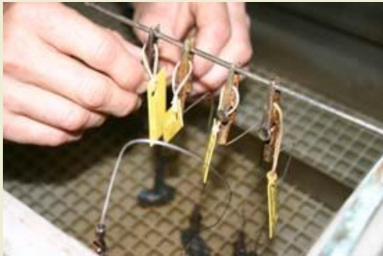
The coins are placed into the electrolysis tanks, beginning the electrolytic cleaning process.
