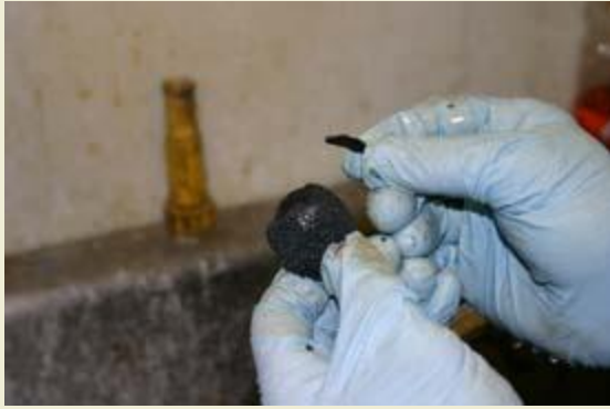
Only a small section of the metal must be accessible to attach the alligator clip.
