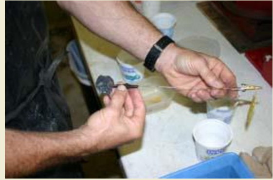
The coin is attached to a stainless steel alligator clip and stainless steel wire.
