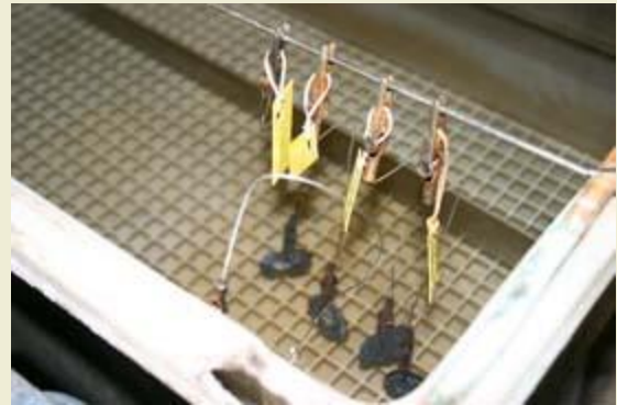
The electrolysis tank consists of Soda Ash and water, with a stainless steel plate (anode) and a low voltage current. During the process of electrolysis hydrogen bubbles are released and the chlorides are expelled from the metal.
